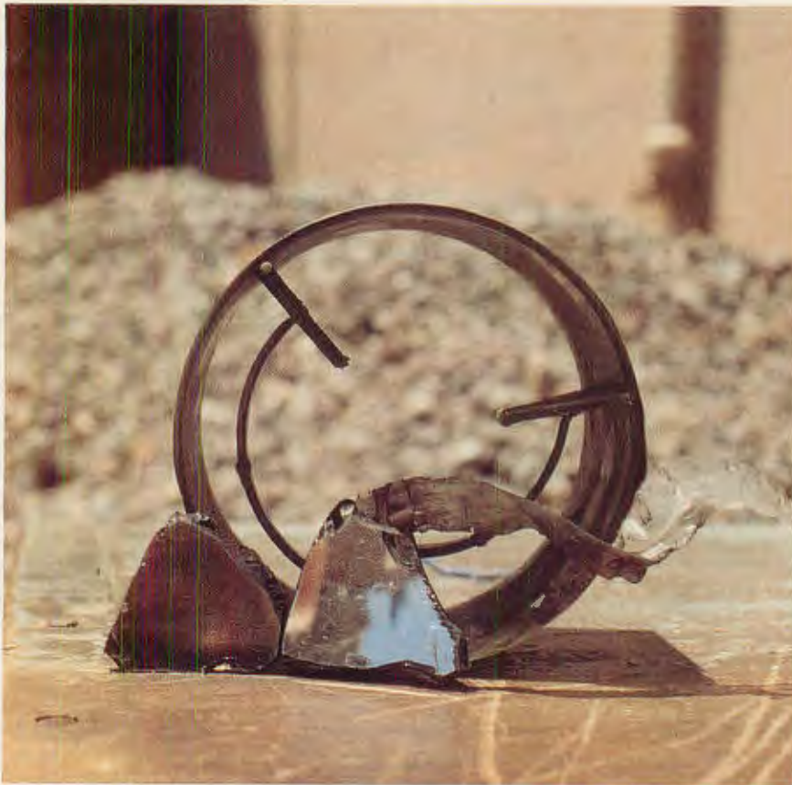
ABOVE: Mirror fragments from mine recovered in the Kabul River. The device behind is a Soviet sensor unit used to command detonate directional fragmentation mines.
